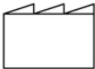
**Customer/Supplier:** In the upper left, generally refers to the supplier where flow begins. In the upper right, refers to the customer (where flow ends).
