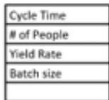
**Data Box:** Goes under process box and contains data relevant to that process step.
