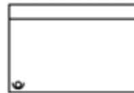
**Process box:** processes through which materials flow. Multiple boxes are used to represent multiple processes in a system.
